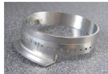
High temperature alloy collar (Haynes® Alloy 25)
